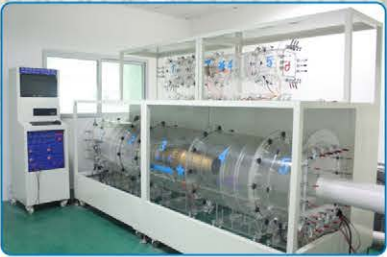
风洞实验室 Windtunnellaboratory One:0~100CFM,0~100mmAq Two:50~2000CFM,0~250mmAq
