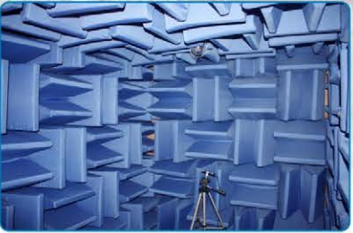
噪音测试房 背景噪音<14.1DB Acoustic Testing Laboratory Back Groud Noise<14.1DB
